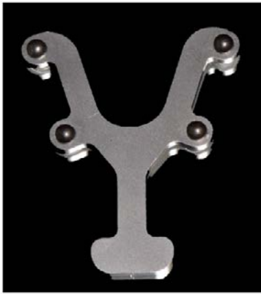
Figure 1. Metallic reference aid with four steel spheres.
